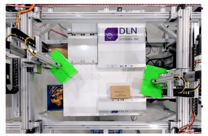
What is the size limitation of products handled? Size and weight of product handled is a wide range. Anything from 6" x 6" up to 36" x 36". However, the size is typically dictated by the size of the tote that the case is being emptied into. The case size being emptied must be smaller than the tote dimension.
